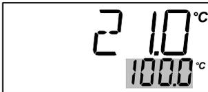
The starting point is the last chosen set-temperature (even if the instrument has been switched off).
