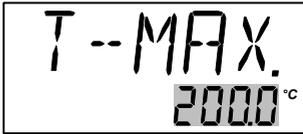
If the current set-temperature is higher than the new max-temperature, you will need to adjust the set-temperature. The instrument will immediately begin to cool (if required) as soon as the new max-temperature is accepted.
