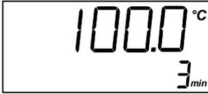
When the calibrator is stable the display will show the ✓ checkmark symbol. The instrument will emit an audible alarm and the estimated time until stable will be replaced by the set-temperature:
