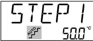
The calibrator will now work towards the given set-temperature. An audible alarm will be emitted once the calibrator is stable. The calibrator will wait the specified amount of extra time. The instrument indicates this by counting down the amount of time remaining:
